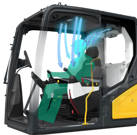
Fig. 12 Air conditioner vent layout
