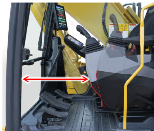
Fig. 9 Left console tilt-up mechanism
