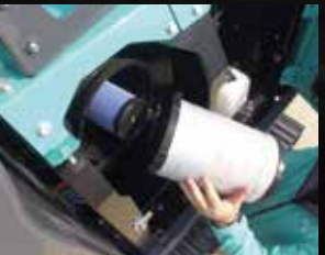
Two-stage air filter
