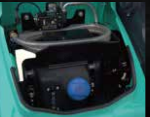
Urea tank Urea filter cap is placed on the step for easy access.
