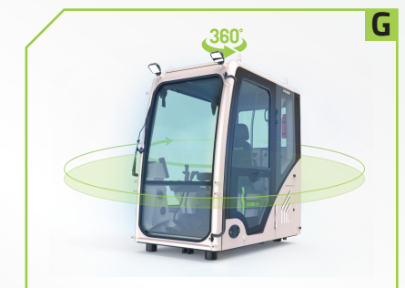
Large-area round view glass glass transmittance increased by more than 11% Sunshade curtain configured as a standard part 大面积环绕式玻璃玻璃通透率提升11%以上 标配遮阳帘
