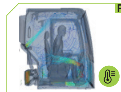
Compared with the previous generation cab, the cooling effect of the new generation cab is increased by more than 19% 新一代驾驶室相比上一代驾驶室, 制冷降温 效果提高19%以上
