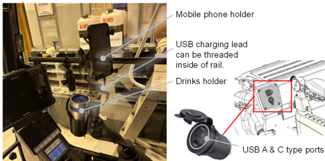
Fig. 6 Accessory rail with USB charger
