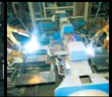
Main frame welding line
