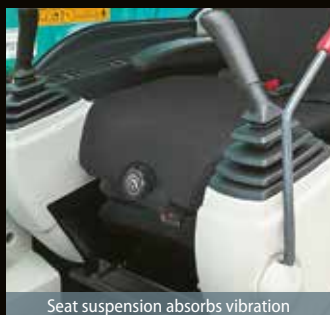
Seat suspension absorbs vibration
