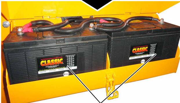
Two 12-Volt Batteries
